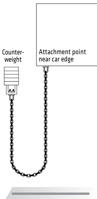
Compensation forms a loop as it hangs from its attachment points. The width of that loop depends on the flexibility of the compensation. Like the materials it replaced, compensating cable forms a fairly narrow natural loop. Note that the compensation is attached near the edge of the car because of this narrow loop.
